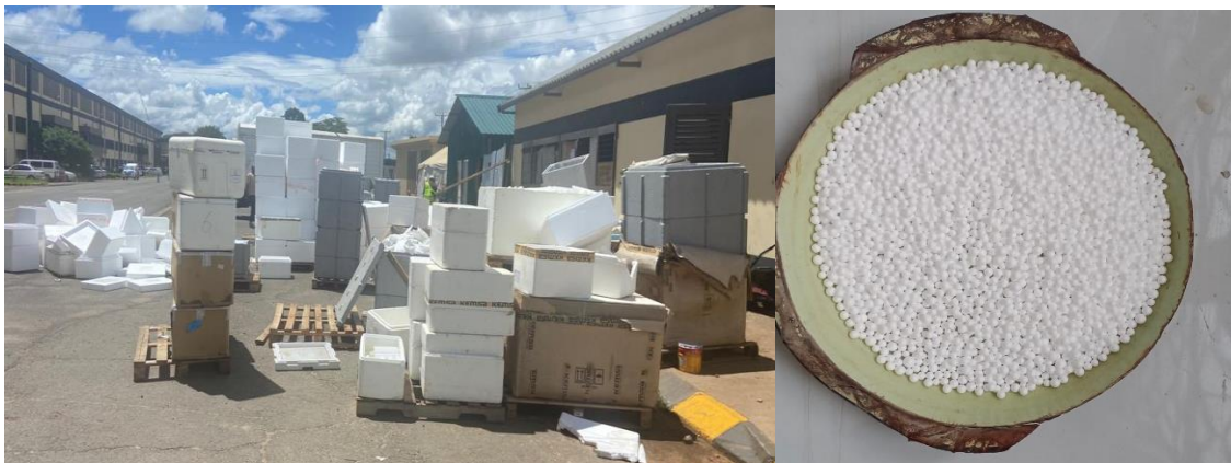
Figure 3.1: Discarded Expanded Polystyrene (EPS) used for transporting good and EPS in beads form
