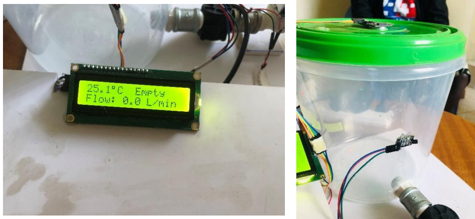
Figure 12. Shows the temperature display operation.
