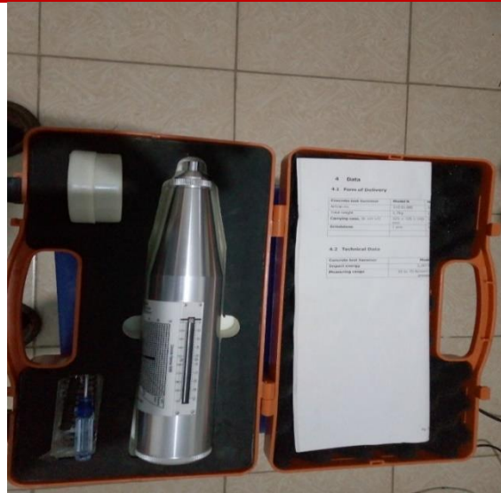
Figure 1: Rebound Hammer used for concrete compressive strength tests (Source: Authors, 2025)
